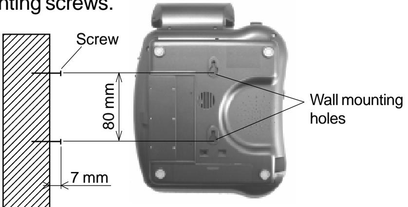
The screws should protrude from the wall by 6-7 mm. Place the phone onto the screw-heads and slide down to secure.
