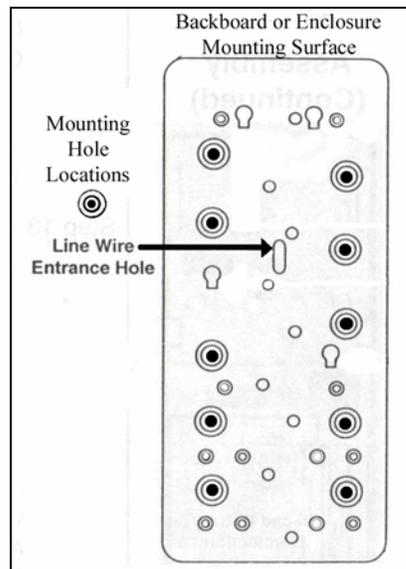
5. Route the telephone line cable through the Line Wire Entrance Hole.
