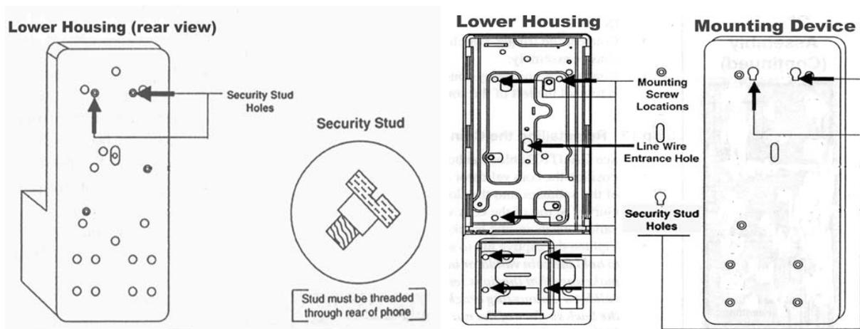
2. Insert the telephone line cable through the line wire entrance hole.
